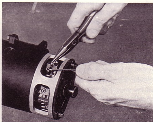
Fig. 42. Removing the brushes
