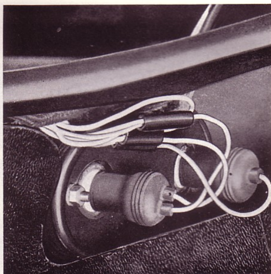
Fig. 90. Rear lamp connecting contacts
