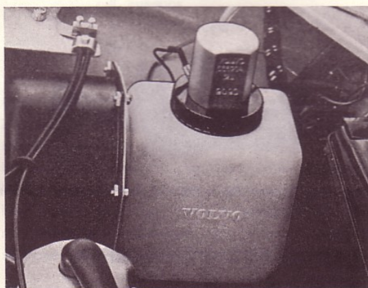
Fig. 103. Windscreen washer, late prod., fitted
