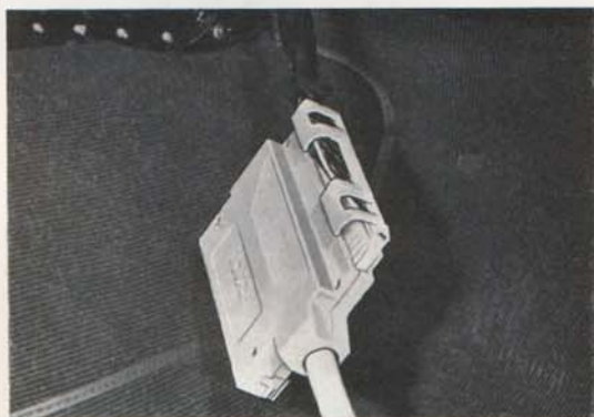
Fig. 2—35. Test instrument connected to the cable harness
