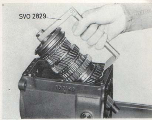
Fig. 4-7. Lifting out the mainshaft
