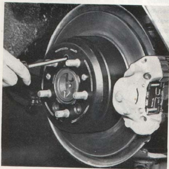
Fig. 5—14. Adjusting the handbrake, rear wheel
