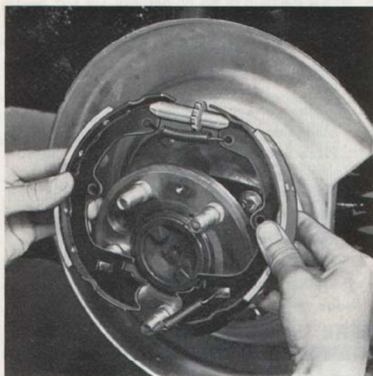
Fig. 5-18. Fitting the brake shoes
