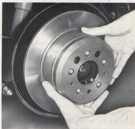
Fig. 5-17. Removing the brake drum
