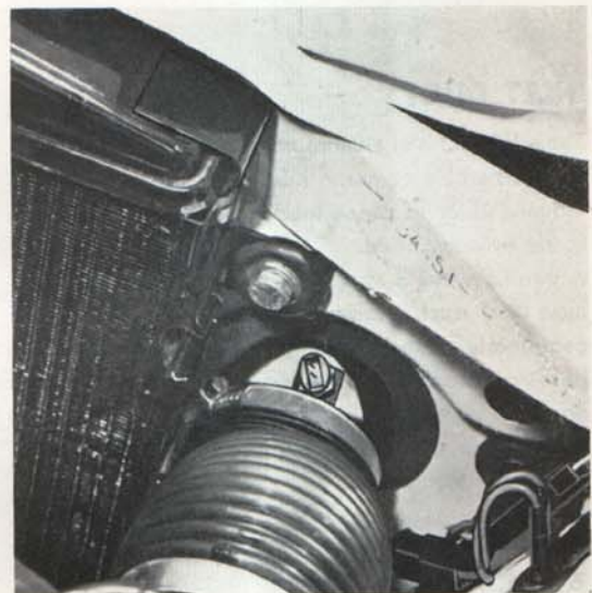
Fig. 2—27. Intake air temperature sensor (connection removed)
