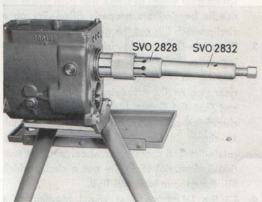
Fig. 4-6. Removing the mainshaft rear bearing
