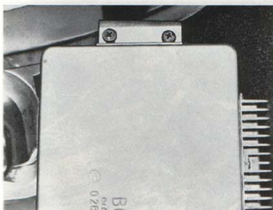
Fig. 2—37. Screws for control unit
