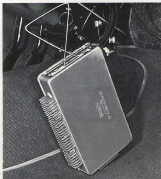
Fig. 2—40. Removing the plug contact
