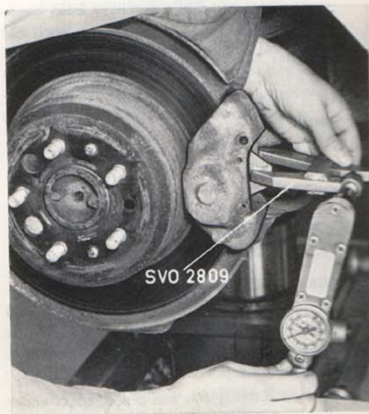
Fig. 5—5. Pressing in the piston
