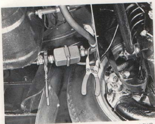
Fig. 2-41. Changing the fuel filter
