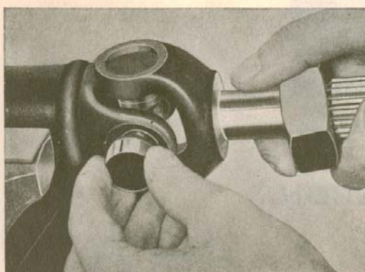
Fig. 4-7. Fitting the joint cross and needle bearing
