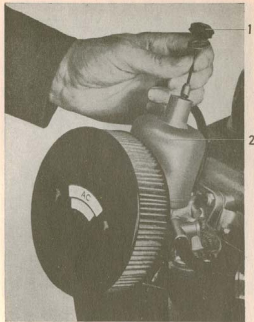
Fig. 1-70. Removing the damping plungers to fill oil in the damping cylinders
