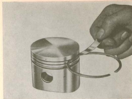
Fig. 1-45. Piston ring clearance in groove
