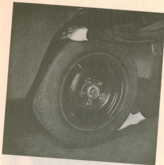
Fig. 8-5. Remove wheel nuts and lift off wheel, taking care to avoid damage to wheel studs
