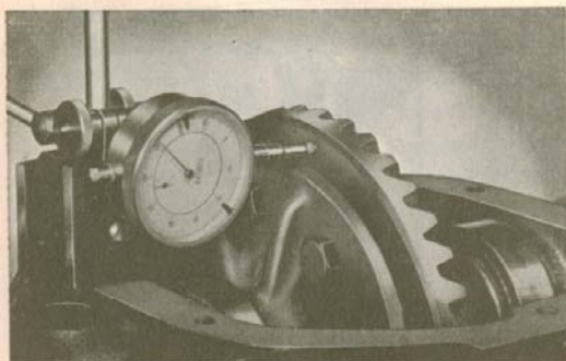
Fig. 5-19. Measuring the differential end play
