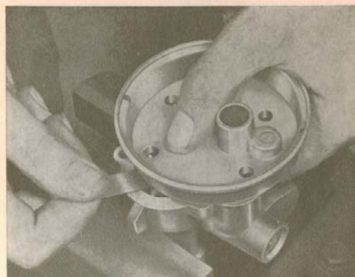
Fig. 1-62. Measuring axial clearance
