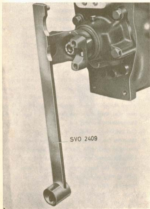
Fig. 3-11. Counterhold for coupling
