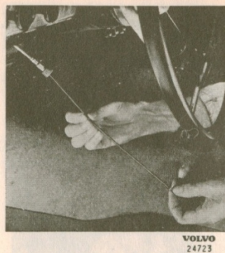
Fig. 12-13. Lubricating the speedometer drive cable
