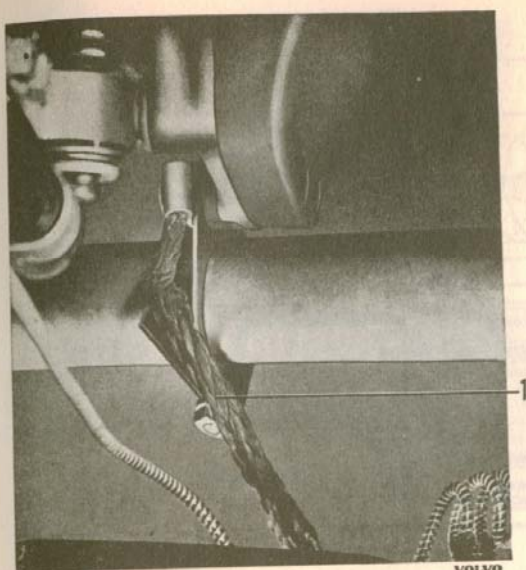
Fig. 10-10. Placing ground lead between engine and body 1. Ground lead
