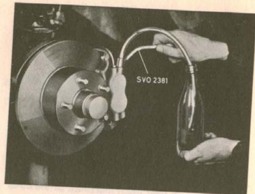
Fig. 7-28. Air-venting (early prod.)
