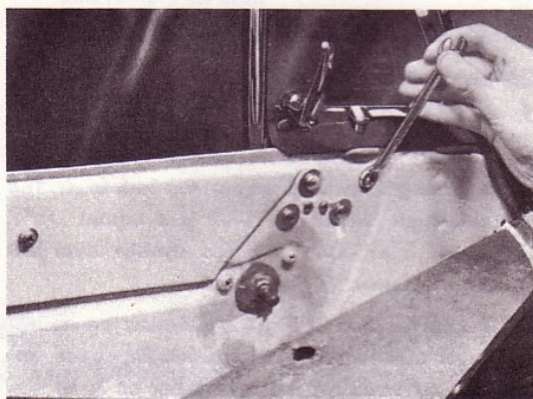
Fig. 22. Removing ventilation window without frame.
