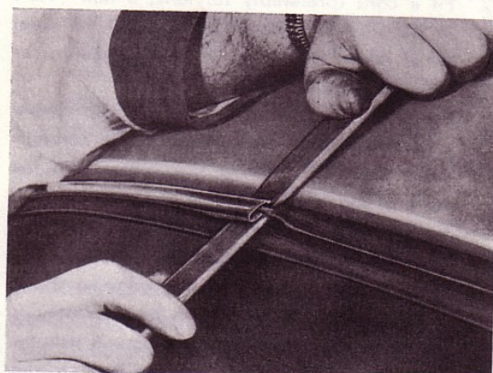
Fig. 34. Removing trim moulding from rubber strip.
