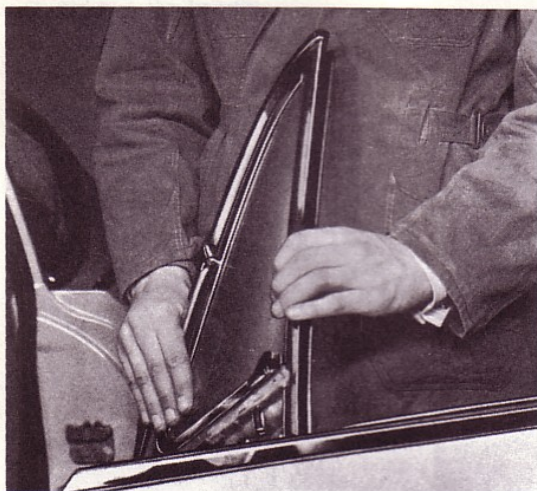
Fig. 20. Taking out the ventilation window with frame.
