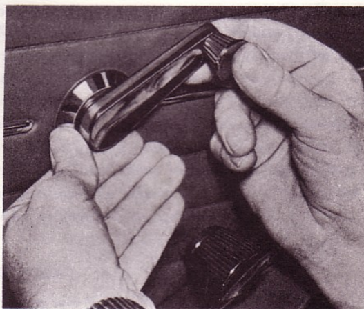
Fig. 7. Removing winding handle, late prod.
