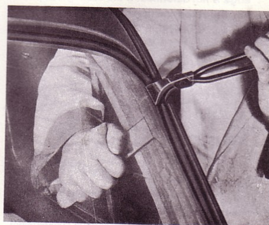
Fig. 37. Releasing rubber strip.
